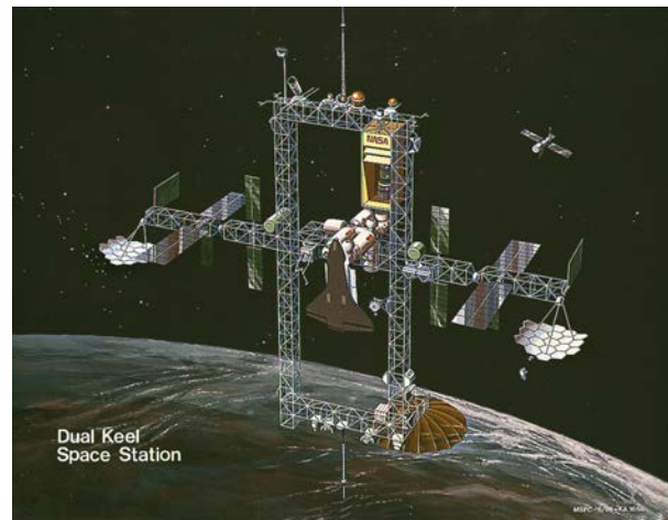
Fig. 17 Artist's concept of Space Station Freedom in its dual-keel configuration (1986) [27]. The modular dual-keel architecture directly influenced Redstar™ .
