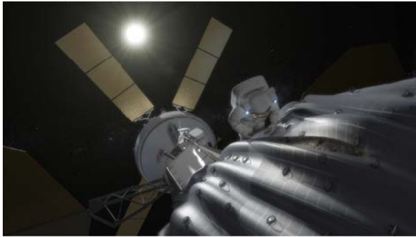
Fig. 1 An ARR option was to deploy a container large enough to capture a free-flying asteroid.
